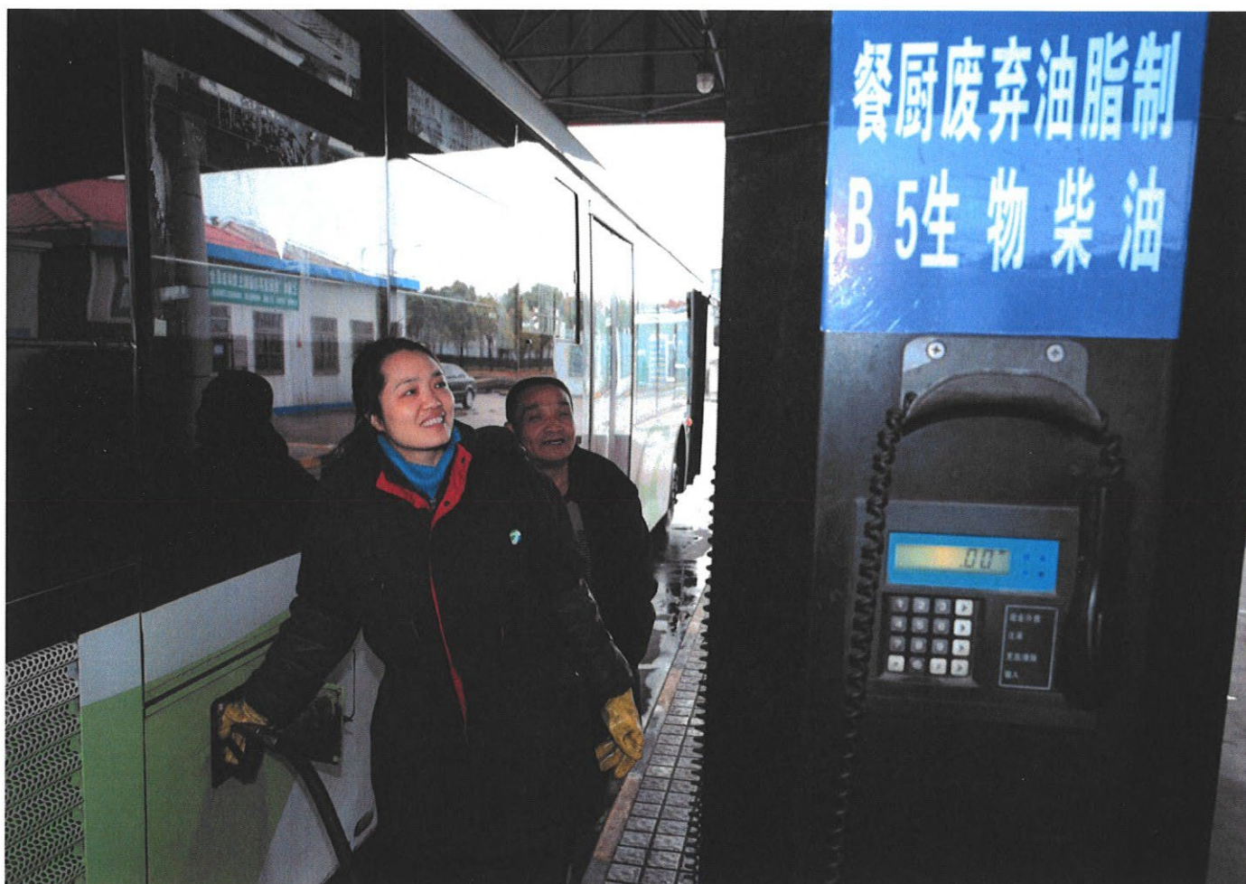
Filling a Shanghai bus with fuel comprised 5% of used cooking oil (Image: Pei Xin / Alamy)
